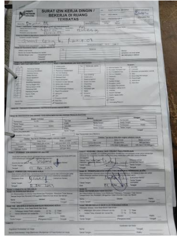
Inconsistency of Permit to Work, no date and for the complete PTW no sign from company man to close
